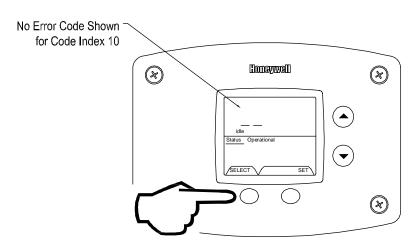
Step 4: Press the "Temperature Down" button to change to the previous code index, code #9.
